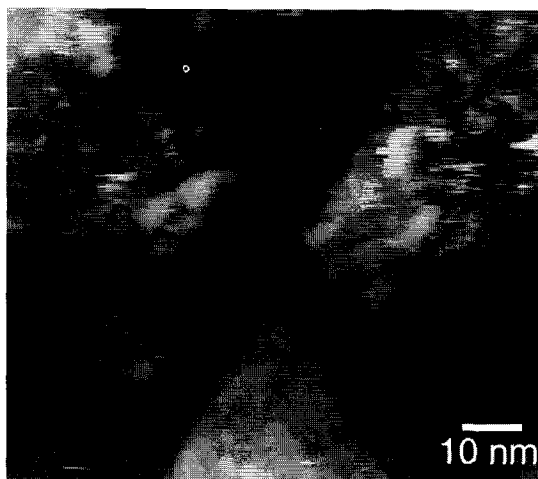
Figure 1: Low-temperature STM topography of a Au (111) substrate covered with a submonolayer of CdSe clusters capped with an organic shell (type I sample). The topography allows the controlled positioning of the STM tip over the clusters to acquire their spectroscopy characteristic.
